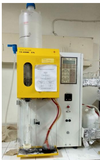
Picture 7: Kjeldahl Analytical set-up
